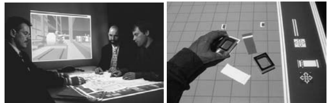
Figure 1: The TUI evaluated is called BUILD-IT. It offers a plan and a side view (left). The system is operated in the plan view using bricks (right).
