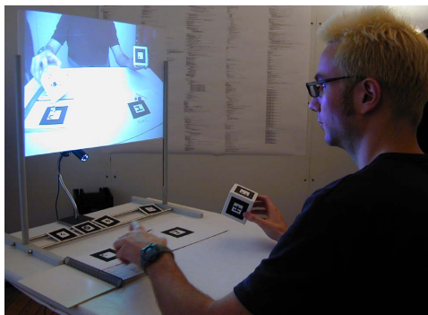
Figure 3: System realization: User charging the gripper with an element from the booklet (left). The platform (right) holds an unsaturated atom, with in close proximity may trigger a binding with the charged atom.
