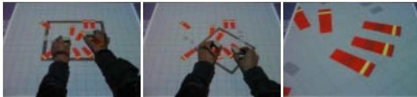
Figure 3: FrameCatcher: Introducing, using, and removing bricks (left to right).
